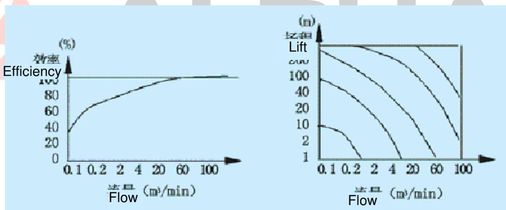
FIG. 2 Efficiency of General Standard Pump FIG. 3 Flow-Lift Characteristic Curve
