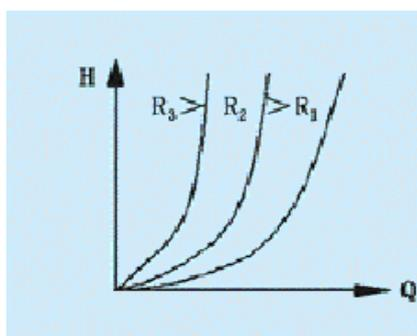
FIG.4 Water Resistance Diagram
