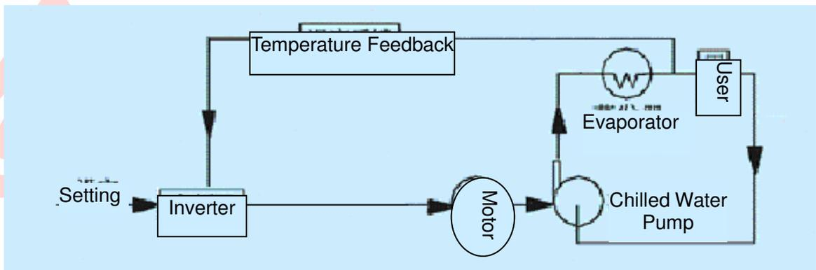
FIG.6 Control Mode of the Chilled Water Pump
