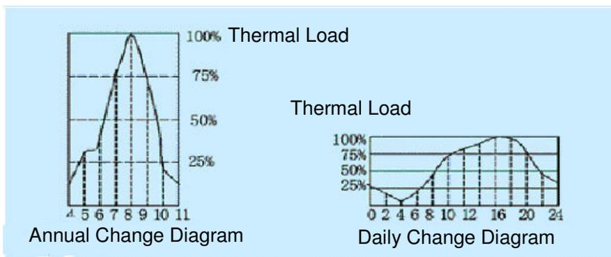
FIG.1 Change Rate Curve of Thermal Load
