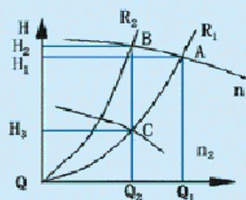
FIG.5 Pump Speed-Regulation and Energy-Conservation Schematic Diagram
