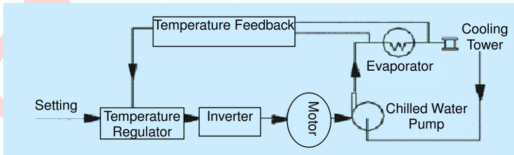
FIG.7 Control Mode of the Cooling Water Pump
