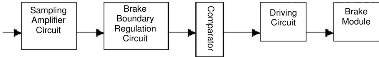
We conduct sampling and amplification of the main circuit, compare it with the reference voltage, and break over the brake unit at  $1.1U_e$  ( $U_e$  refers to the rated bus bar voltage value) and turn it off at  $1.05 U_e$  through regulation of the potentiometer. In this way, voltage of the main circuit can be controlled to ensure it operate within the permitted range.
