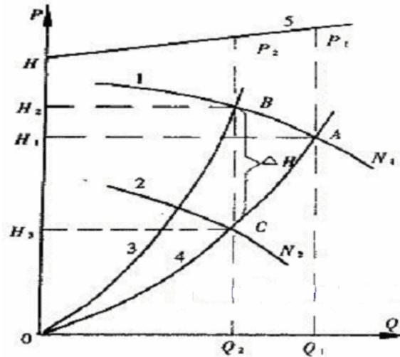
FIG. 2 Performance Curve of the Fan during Frequency-Conversion Regulation
